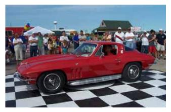
Visually, the easiest way to tell a 1965 Corvette from a '64 is the three functional vertical louvers in each front fender. But the big news (literally) was the availability of the new 396-cubic-inch big-block V8. And there was even better news as four-wheel disc brakes became standard (though 316 fools did delete them in favor of drums and a \$64.50 credit).
