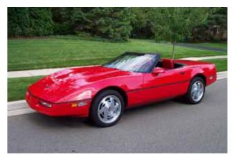
New 17-inch wheels inside P275/40ZR17 tires were added to the 1988 Corvette options list while new aluminum cylinder heads and a revised camshaft boosted the L98 to 245 horsepower with even better torque characteristics. This was also the last year Chevy would foist the dreadful 4+3 transmission off as the shift-it-yourself choice. A 35th anniversary model, done in a white-on-white scheme, marked this milestone.
