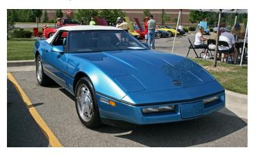
In 1988, Corvette started using a unidirectional 17" wheel as an option with RP0 Z51 and Z52. New six slot 16x8.5 were standard with P255/50ZR1 Tires.
