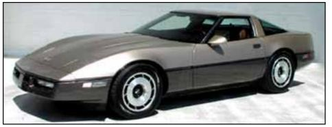
One styling element that was new to the C4 Corvette was a full-perimeter rub strip at roughly mid-body height. This not only tied the front and rear bumpers together visually but concealed the one major seam in the new bodyshell, as well as the shutlines around the clamshell hood.
