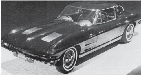
Designer Larry Shinoda was given project and stretched the already penned 2-seat midyear coupe to accommodate the back seats and the extra legroom required. Six inches was added to the C2's wheelbase to stretch it out to 104 inches. The pictures below show that the four-seater Corvette's doors are much longer and shaped differently than the production 2-seater. The roof is also slightly taller and the rear glass looks to be longer as well.
